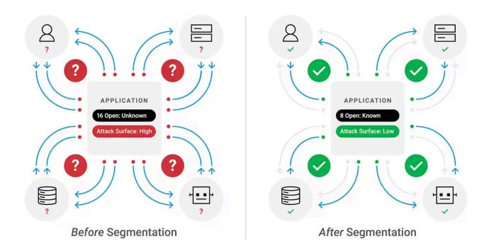
Software-defined microsegmentation is a network security technique that splits or segments a network into extremely granular areas, allowing individual workloads, applications, and virtual Diagram illustrating network segmentation.
